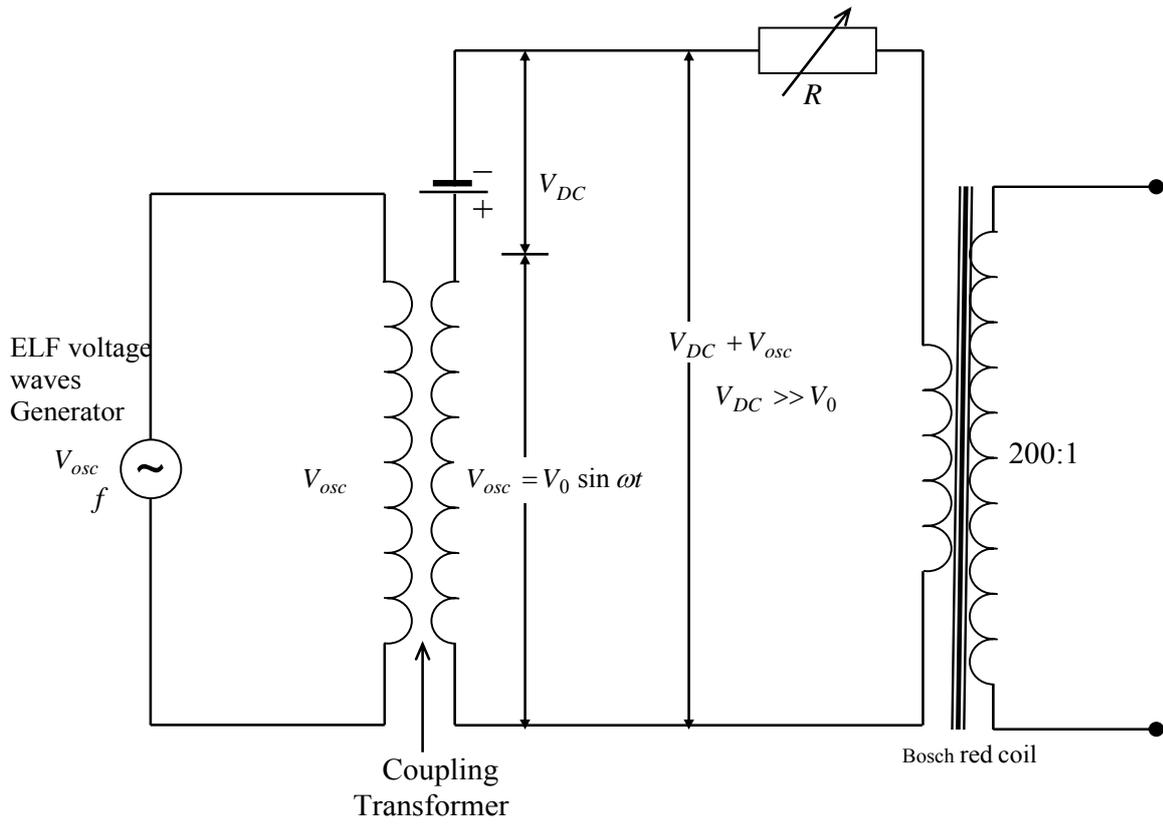
Fig. B3 – Equivalent Electric Circuit
