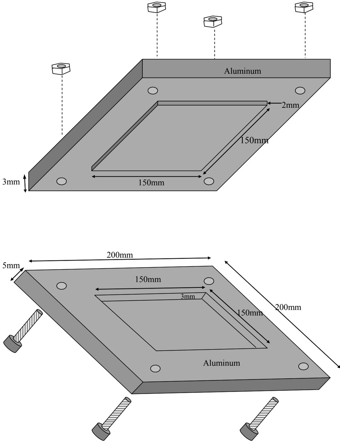
Fig.B1 – Mold design
